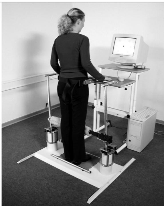
Fig. 4. A photograph of the BalanceReTrainer prototype and a neurologically intact individual exercising computer based balance-training task.
