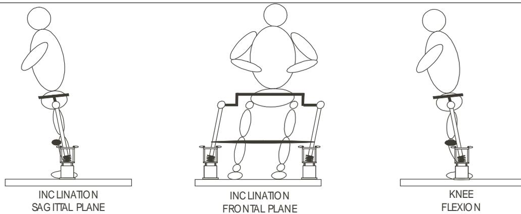
Fig. 2. Schematic presentation of the three DOF of the apparatus (inclination in the sagittal plane, inclination in the frontal plane and movement along the vertical postural axis – knee flexion/extension).
