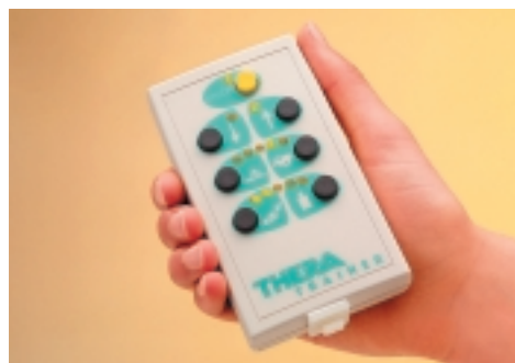
Direction of rotation, speed and resistance are adjusted by the infra-red remote control.
